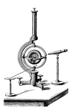
Foucault's gyroscope. Once the central, doughnut-shaped rotor had been set spinning, its axis remained fixed in space. The resultant motion of the low-friction gimbals was a reflection of the Earth's rotation and could be monitored with the pointer or microscope.
