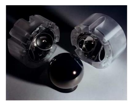
The GP-B gyroscopes are 38.1-mm diameter quartz spheres covered with a 1.27- $\mu$ m layer of niobium. Their sphericity is only some 40 atomic layers from perfect. Only neutron stars are rounder.
