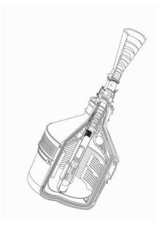
Cutaway of the Gravity Probe B payload. The main vessel or dewar (lower) held an initial charge of 2400 litres of liquid helium coolant. A tube along the central axis holds the quartz gyroscope housings and a 142-mm telescope, which points through the neck of the dewar and through the conical sunshade (upper) to track the guide star. GP-B was launched into a polar orbit of 642 km altitude from Vandenberg Air Force Base on 2004 April 20 by a Delta II rocket.
